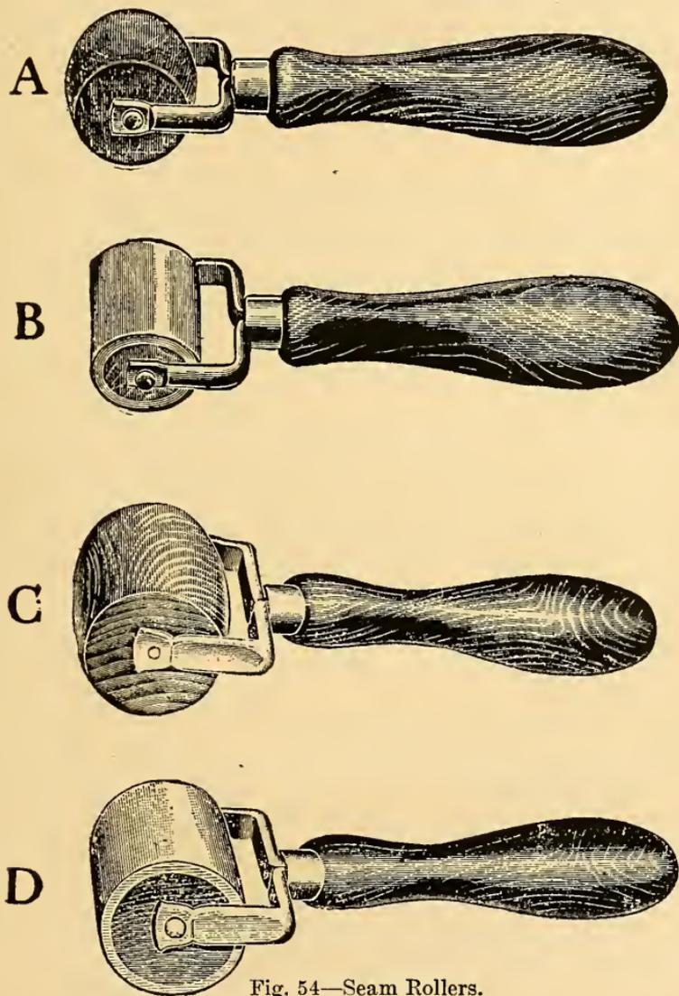
Fig. 54—Seam Rollers.
