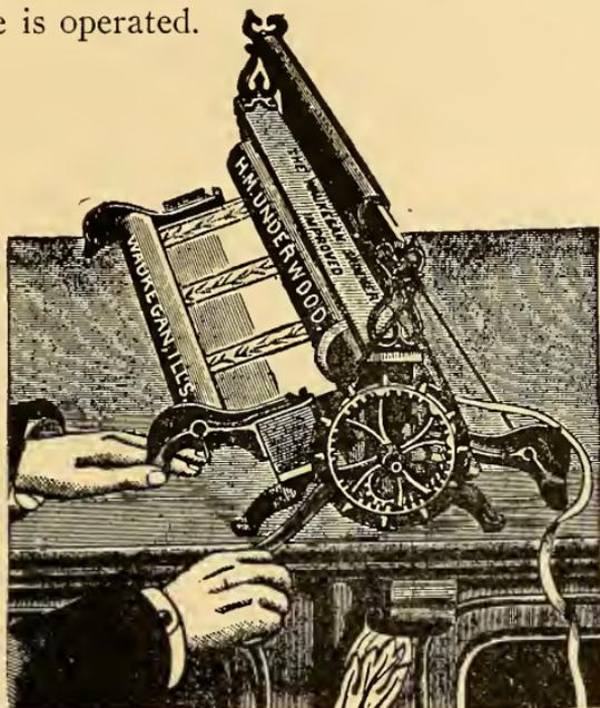
Fig. 59—Machine Trimmer.
